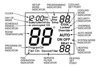
Fig. 1 — Thermostat Display
